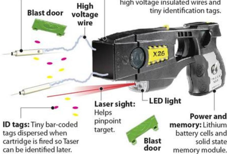
**Taser range:** X26 can hit target up to 10.6 metres (35 feet) away.
